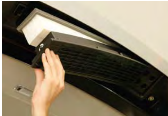
Two externally accessible cab air filters are easily changed and keeps the cab interior free of dust.
