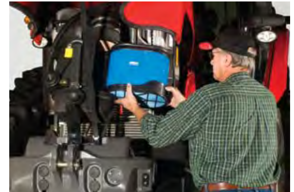
All 8600 Series models feature a new cassette type engine air cleaner, positioned at the front of the tractor, making service even less time consuming.
