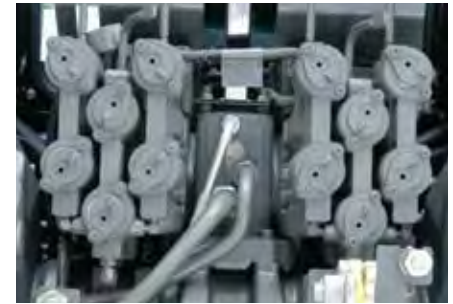
Implement hook-up is fast and easy, thanks to decompression couplers that allow hoses to be connected and disconnected under pressure.
