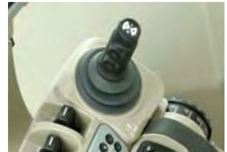
The joystick is especially valuable for faster, more efficient loader work or when performing complex equipment commands during headland maneuvers.
