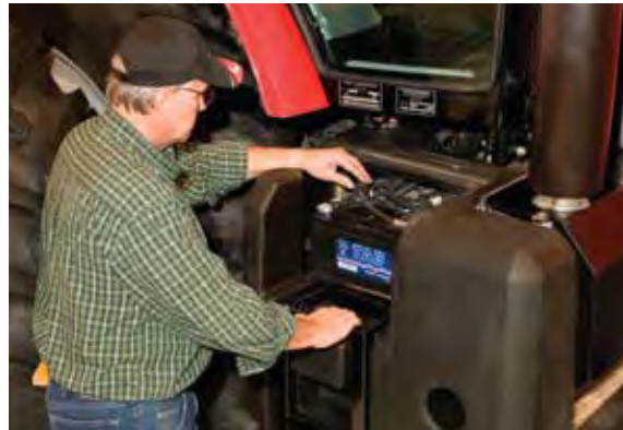
The batteries are easily accessible by removing a cover beneath the steps on the right side of the cab.
