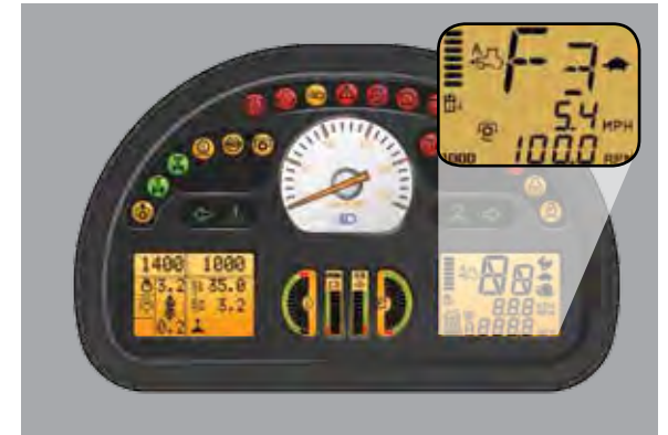
Hydraulic and powertrain oil indicator in the Dash Control Center of the tractor let you check the level at a glance.
