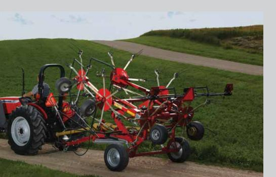
even offers a choice of two 25-foot models, including the TD1648, which incorporates its own transport chassis that allows the rotors to fold forward and rest on rubber dampers for high-speed transport between fields.
