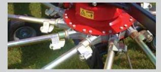
A FULLY ENCLOSED GEARBOX on each rotor prevents contamination from dust, dirt and debris for maximum reliability. The helical-cut gears and sealed cam track are also permanently lubricated with grease, rather than oil, to prevent leakage and increase service life.
