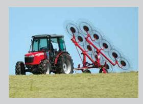
**ONE SINGLE-ACTING CYLINDER** folds both wings for easy transport.
