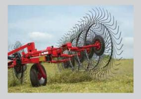
**ADJUSTABLE FLOAT SPRINGS** on each rake arm let the operator select just the right amount of down pressure for the crop and field conditions.
